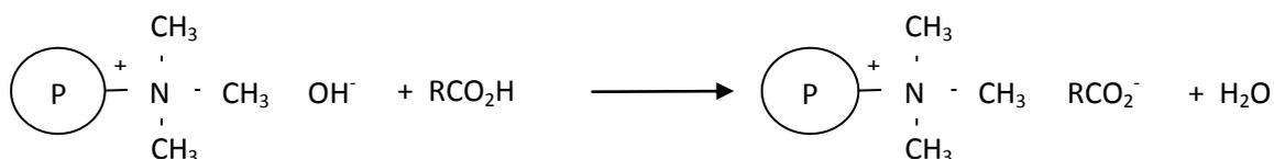
The salt of fatty acids produced by the reaction is fixed on the resin and the water that is released during the reaction can be evaporated by heating the oil. The resin with fixed salt of fatty acid can be separated from the oil by filtration or centrifugation. The resin can be regenerated by washing with a solution of mineral acid like hydrochloric acid or sulfuric acid followed by a washing with a solution of sodium hydroxide.
