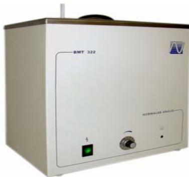
Copper strip corrosion apparatus
